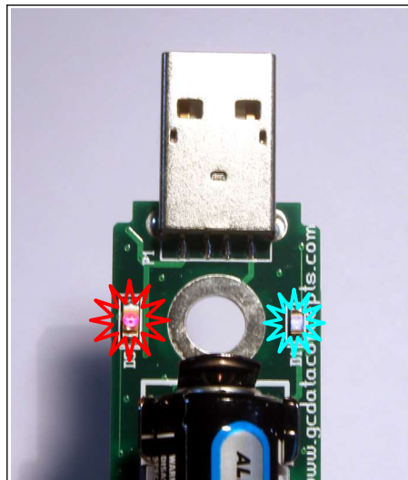
Figure 13: LED Status Indicators
